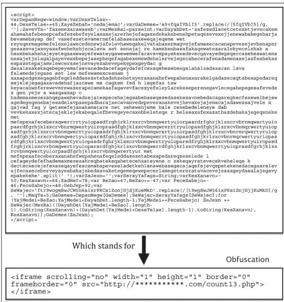
Figure 3 Obfuscation used in JavaScript code
